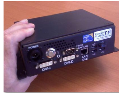
THERMAL MATRIX IP-500 is ultra small and lightweight, measures 7"x 5.5"x 2.5"
